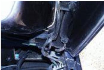
08: Now you can remove the headlight. Locate the clip that holds the wires to the headlight frame - it should be located in the corner of the frame. Remove this clip with a small flat-blade screwdriver by carefully prying it off. Once the clip is removed, unweave the wire from the support and remove the motor assembly from the car.
