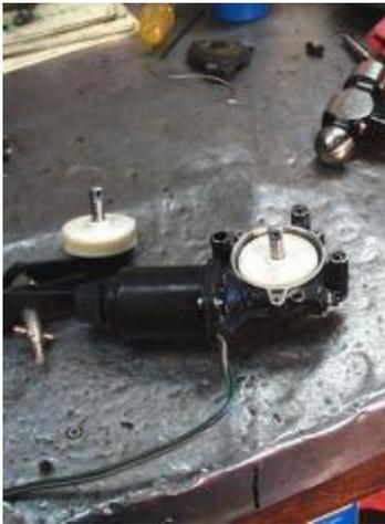
19: Now reinstall the gear into the housing, and reverse the disassembly to reassemble the headlight motor and linkage. Once they are back together, use the manual knob and completely rotate the headlight through its full cycle to make sure it does not bind. If it does bind, you probably put the little stop bracket between the motor and the linkage on backwards. Once the headlight works manually, set the linkage back to the closed position and reinstall the motor into the car.
