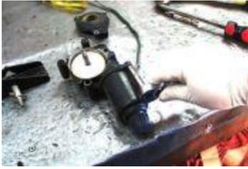
12: Now very carefully loosen - but do not remove - the pair of motor housing screws. If you remove them you could permanently damage the motor.
