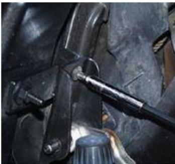
06: Using the Torx socket, remove the motor bracket screws that attach it to the headlight support.
