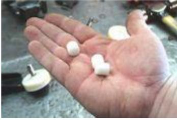
17: Here are the new bushings supplied by [Zip Corvette](#) for the rebuild. The headlight motors use three bushings per side.
