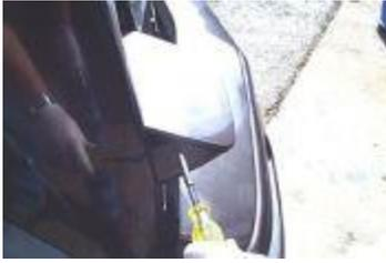
03: Rotate the headlight until you can see the screw that holds the sides of the headlight bezel. Remove it along with the two Torx screws in the front of the bezel.
