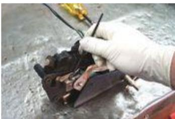
09: With the motor out, start disconnecting the motor from the linkage assembly. Use a small punch to remove the roll pin from the linkage where it connects to the motor shaft.
