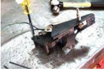
10: Use the Torx bit to remove the three screws that hold the linkage to the motor itself, then you can remove the motor from the linkage. There is a small stop that rotates with the motor and linkage, make note of its location and how it is mounted so you can reassemble it in the same manner.
