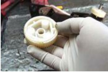
18: Place the three new bushings in the gear, then press the aluminum housing over the top of them. It will be a very tight fit.
