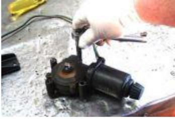
11: Remove the small 1/4-inch screws that hold the gear cover on. Once they are out, the cover will come off by gently prying on it.
