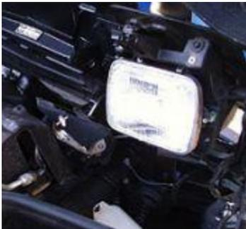
07: Once the Torx screws are removed, the headlight motor will pull away from the housing and frame. Before you remove the motor from the housing, rotate the headlight to the closed position. Also, note the location the linkage assembly because you will need to reassemble it in the same location.
