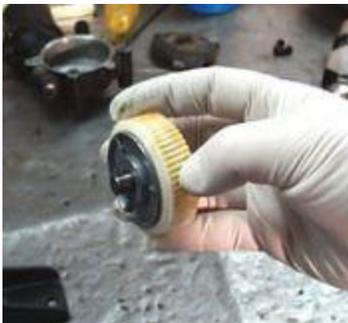
15: Once the gear is out, you will see a nylon gear and the aluminum housing the gear sits on. Press the center shaft while holding the nylon gear. This should separate the aluminum housing from the nylon gear.
