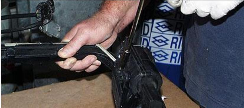
If you look at the side of the headlight motor, you will notice a small bracket that bolts to the headlight frame and the hood hinge. Unbolt the 13mm carriage bolt between the bracket and the hood hinge, then remove all of the 10mm bolts that hold the headlight motor to the headlight frame. Then you can remove the motor.
