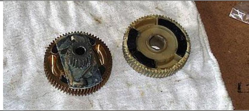
In a side-by-side comparison, you can see the difference between the bronze gear (left) and the original nylon gear. The new bronze gears won't wear out like the originals.
