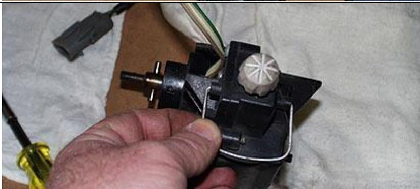
With the motor out, remove the wire clip from the locking knob. Just pull it out of the housing.
