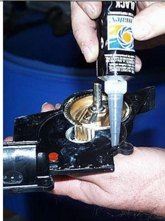
Before bolting the two halves back together, you will need to apply a small amount of silicone sealant to one of the halves to prevent water from shorting out the motors. Then reassemble everything in the opposite order that you removed it.
