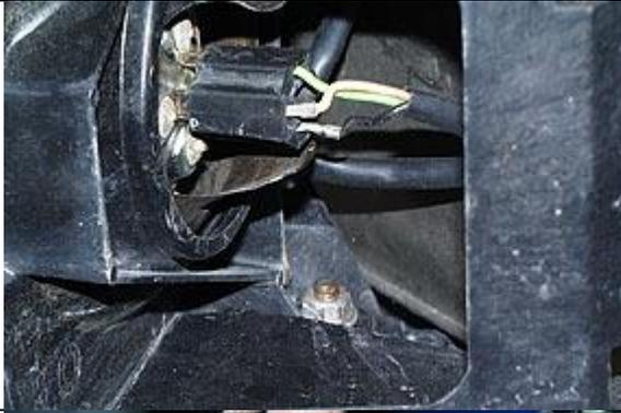
Looking into the headlight housing towards the location of the headlight motor, you will see a retaining nut. Lubricate it with WD-40 before removing it with a 1/4-inch ratchet with a long extension and 13mm deep well socket.
