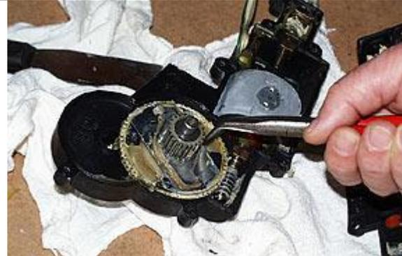
Using a pair of needle nose pliers, pull the main (large) gear out of the motor housing, then pull up on the metal gear and it will slip right out. Remember how this gear is assembled because you need to reassemble the bronze gear the same way. If you happen to receive a bronze gear without the rubber pads in it, just reuse your original ones. Once you have the gear assembled, apply a liberal amount of lithium grease to the entire gear and reinstall it into the motor housing.
