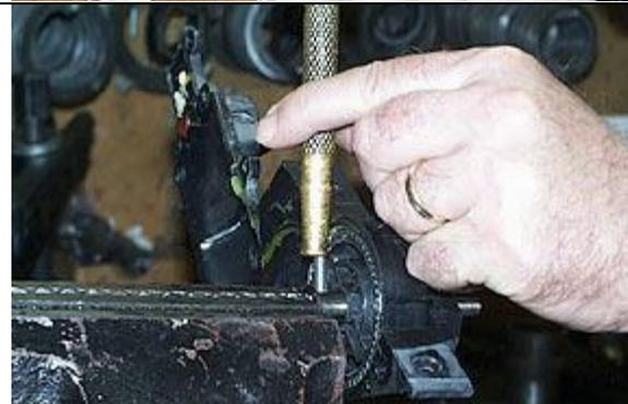
For the small gear, you will need to lock the shaft into a vise. Then use a brass punch and hammer to remove the pin that locks into the gear.
