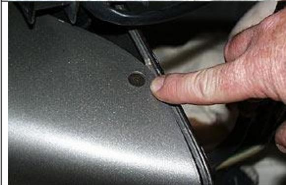
This is the side screw we are going to remove. This is a special screw so make sure you do not misplace it.
