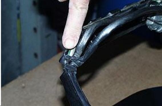
Locate the metal wire retaining clip located in the corner of the headlight frame. You need to carefully remove the clip so that it does not go shooting off somewhere in your garage. To remove it, gently pry up on the small prongs and the clip will slide off. Once the clip is off, remove the headlight motor wires from the headlight frame.
