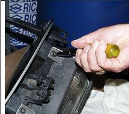
With the side screws are out, remove the front Torx screws, then separate the headlight cover from the headlight housing. Remember to lay it on something soft because you do not want to scratch the paint.
