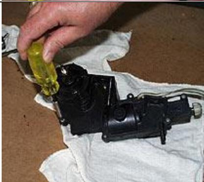
Use a Phillips screwdriver to remove the screws that hold the housing together. Silicone sealer was used at the factory to keep water out, so you may need to use a small putty knife to separate the housing.
